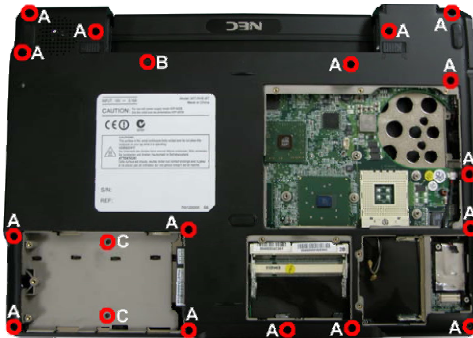
Fig. 18 Removing the top cover screws
